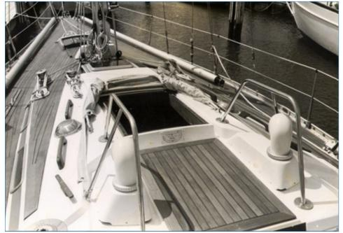
Cockpit: Although small it is highly functional. The helmsman is particularly cared for with a seat and a floor with angled foot rests. The starboard longitudinal seat opens completely for access to the life raft. Note the Tannoy vents for galley and head respectively, the teak handrails and the three-legged grabrails assisting the companionway user, the small dodger over the entrance providing protection in hard weather or rain, and the well shaped cleats properly located and sized.
