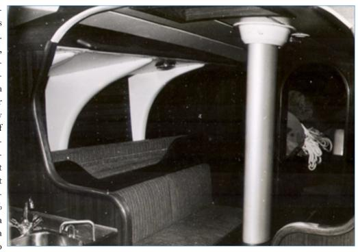
The saloon: With two berths each side it is perfectly symmetrical. The folding table can take six persons, but this blocks the passage to the bow. The mast in the middle sometimes hides the face of the tablemates, but provides a very good support when moving around. Behind the seat backrests six deep stowage lockers. Note the stainless tie rod connecting the deck to the keel.
